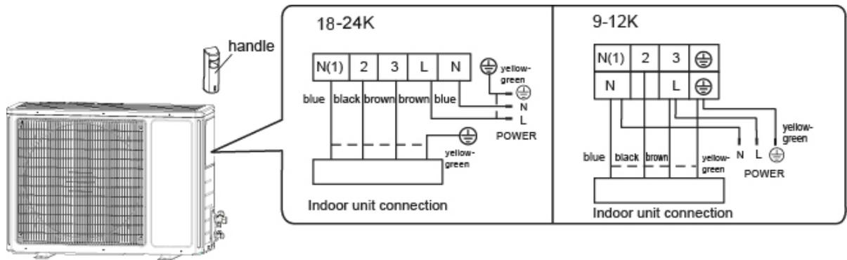
2. Secure the power cable and the signal control cable with the clip (only for cooling and heating units).
