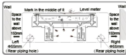
Drill a piping hole of diameter  $\Phi 55$  at the chosen location for the outlet pipe. To allow for proper drainage, the piping hole in the wall must slant slightly downwards to the outdoor side, with a gradient of  $5 - 10^\circ$ .
