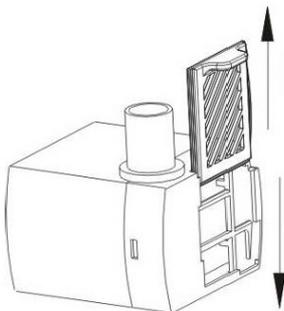
Prior to starting maintenance operations, make sure that the appliance is unplugged. The filter must be kept clean to ensure optimal operation of the appliance. If the filter is clogged or water cannot pass through it, clean it as shown in the picture.
