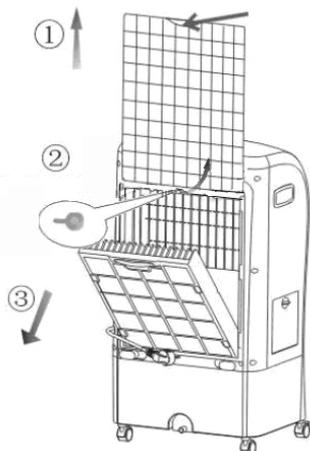
Pull the tab upwards. Turn the upper knob upwards as shown in the picture. Lift the filter by pulling it upwards.
