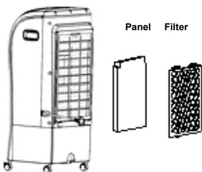
Clean the dust filter using a soft brush or vacuum cleaner, and wash it in water containing a neutral detergent. Remove the cooling panel as well and soak it in water containing a neutral detergent. Extract the tank and rinse it under running water, while removing any residues. Let the filter, panel and tank dry fully after they are washed, then re-mount the components in the following order: water tank, cooling panel and dust filter.
