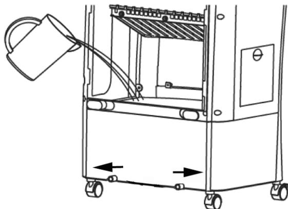
Counter-rotate the tank knobs by 90° and remove the tank from its housing; fill it **with demineralised water** up to the maximum level mark. Replace the tank into its housing and turn the knobs.
