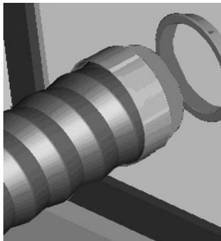
5. Insert the flexible pipe thus mounted into the rear of the air conditioner.
