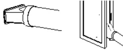
3. Open the window and lock one of the two leaves with the handle. Rest the terminal connection on the fixed leaf, bring the other leaf of the window close.
