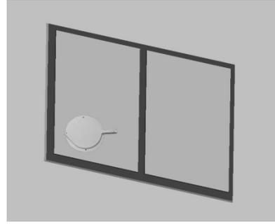
3. Insert the round fitting into the retractable flexible pipe and insert the latter with its round fitting into the window unit without the plug.
