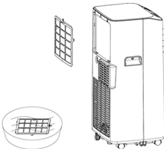
The air filters must be checked at least once every two weeks of use. Operating the appliance with dirty or clogged filters will decrease the air conditioner's efficiency and may cause serious problems.
