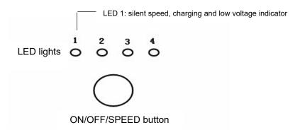
**ON/OFF/SPEED button:** Press this button to turn on or turn off the fan and to switch the ventilation speed sequentially: Silent (LED 1) -> Low (LED 2) -> Medium (LED 3) -> High (LED 4) - >OFF
