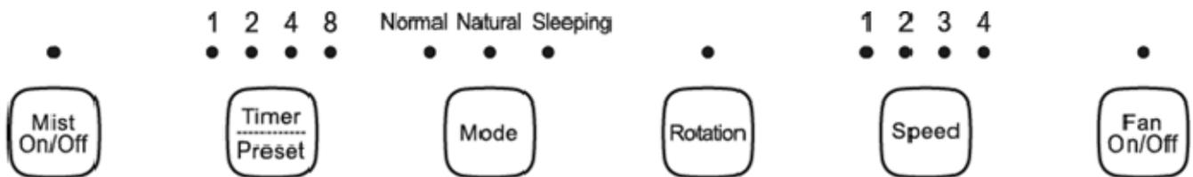
**All the buttons on the control panel are touch-sensitive: a light touch is enough to select the functions.**
