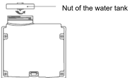
Reposition the tank in its seat and close.
