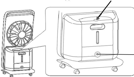
Plug to be unscrewed to drain the water generated by the humidification process
