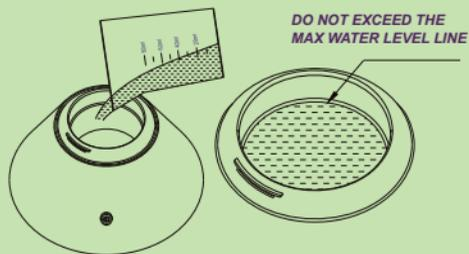
2. Fill the water tank with clean water (Maximum 80ml.)
