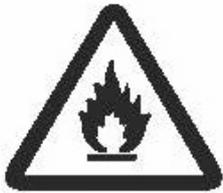
Appliance is filled with flammable gas R290.
