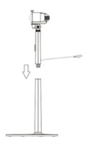
2. Fix the Control Box (Upper Stand Tube) into Lower Stand Tube, screwing it.
