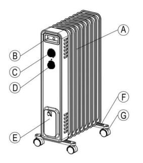
A. Heating elementsB. Integrated carrying handleC.Thermostat knobD. Power switch knob
