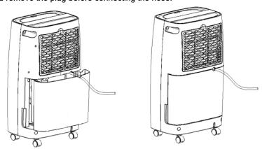
Remove the tank and safely connect the hose to the continuous condensate discharge connection, as shown in the figures below.
