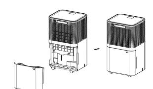
Do not use the dehumidifier without the filter as dust may affect the efficiency of the evaporator, resulting in higher energy consumption.
