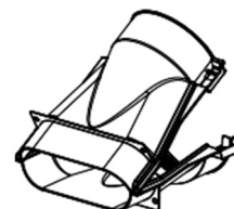
End fitting for window, supplied into 2 parts to be joined with 2 tabs that fit together. (2)
