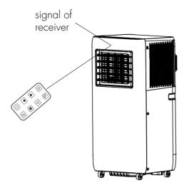
Make sure to direct the remote controller towards the signal receiver located on the front of the appliance, as shown in the figure.
