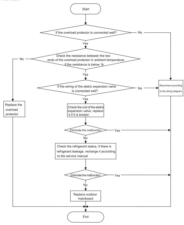
Note: the detection method of the coil of the eletric expansion valve: there is five pieces of coil of the eletric expansion valve, the resistance of one of them (the leftmost or the rightmost one) is almost the same as the resistance of other terminal (within  $100 \Omega$ ). Judge the condition of the electronic expansion valve through detecting these resistance.
