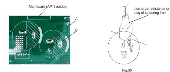
(3) After finish discharging electricity, measure the voltage between point A and B with universal meter to make sure if electricity discharging is completed, in order to prevent electric shock. If the voltage between the two points is below 20V, you can perform maintenance safely.
