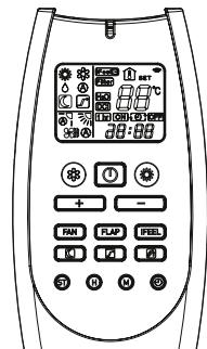
At this point, press contemporary the FAN and IFEEL keys of the remote control for more than 5 seconds and release them by pointing the remote control towards the indoor unit.
