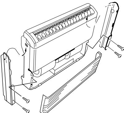
**EG** Fix both side panels and reassemble the return air grille.
