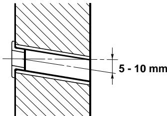
**EG** Drill a hole (see table), insert a PVC pipe, fit the plastic cover supplied with the unit.
