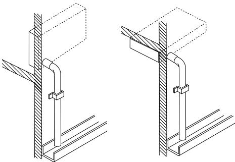
**EG** Install the condensate drain to the outside with a positive slope.
