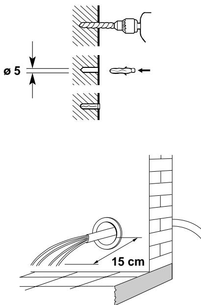
**EG** Predispose the fixing of the bracket. Running power electric cable (with a ground wire) between the two units (see the table of wire section). Check if the quantity and the rawl plugs type supplied are the proper ones for fixing the unit on the wall.
