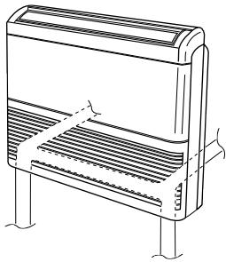
**EG** Find the place for the installation. The unit can be connected in four different positions: at the right-back side, at the left-back side, at the bottom on the right or on the left.
