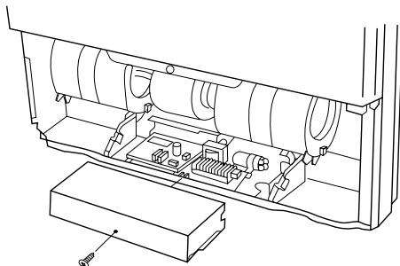
**EG** Remove the electrical box cover to operate on the terminal strip.
