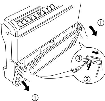
**EG** Remove the return air grille releasing it from the side guides and the central elastic stop.
