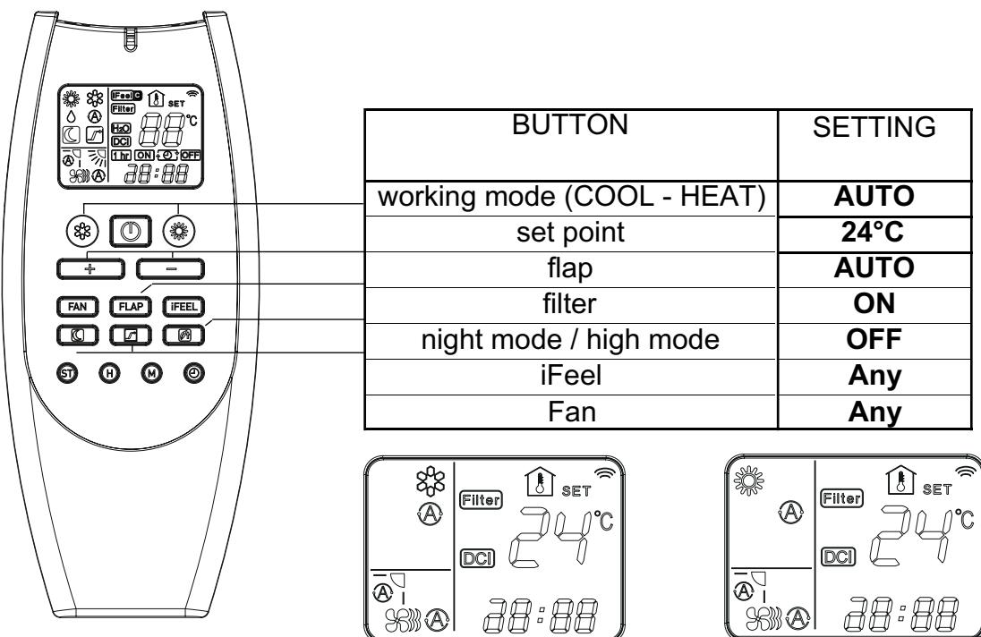
Press together FAN + IFEEL buttons for more than 7 seconds and release them pointing the remote controller to the indoor unit receiver. Be sure to send the signal to only one indoor unit and that there is no other indoor unit that could receive the same signal.
