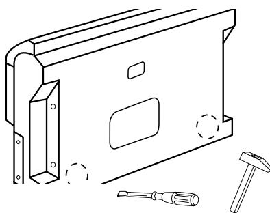
**EG** Open a pre-punched hole for the pipe passage (work from outside).
