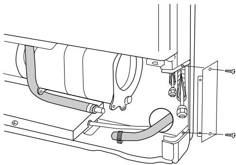
**EG** Remove the side panel to operate on the connecting pipes. Predispose the condensate drain pipe and attach it to the fan housing if necessary.
