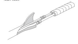
Air purging of internal unit and refrigerant tubes. Connect the vacuum pump to the outside unit as shown in the figure. Air and moisture have undesiderable effects on the refrigerant system.
