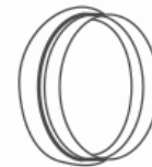
Round fitting for window unit, for positioning between the end of the tube and the window unit itself.
