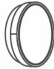
Round fitting for window (1) to be positioned between the end of the tube and the end fitting for the window
