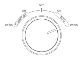
Place the selection knob in the desired position: ECO "ON" (400 W) or COMFORT "ON" (800 W).
