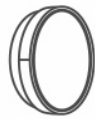
Fitting to apply on the unit to which connect the exhaust pipe of the air
