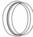
Circular fitting for kit porthole to be positioned between the final part of the tube and the porthole
